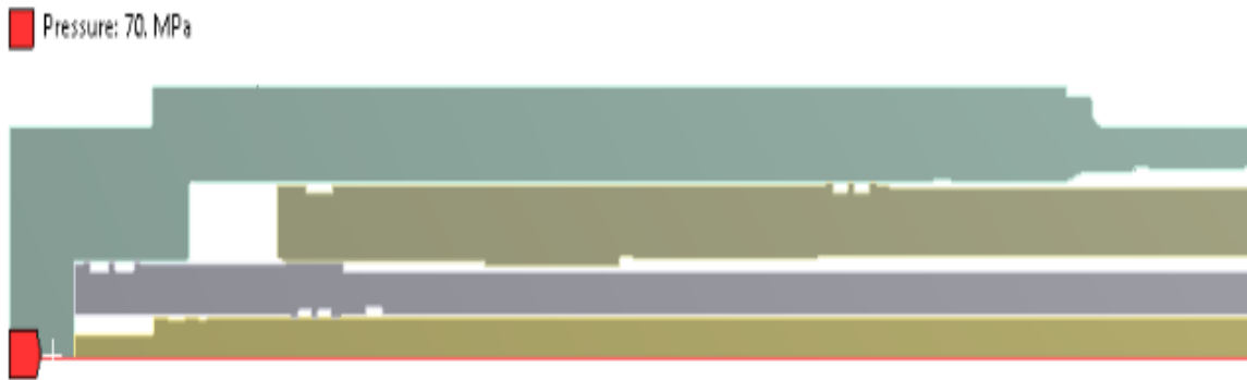
Figure 7: Pressure at the tubing inner surface
